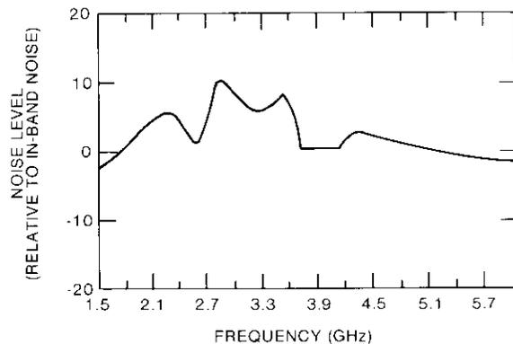
Figure 1. LNA Noise Output Relative to In-Band Noise
