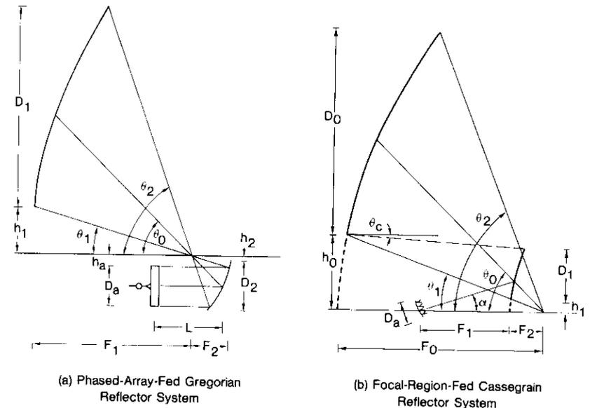
Figure 2. Phased-Array-Fed and Focal-Region-Fed Dual-Reflector Systems
