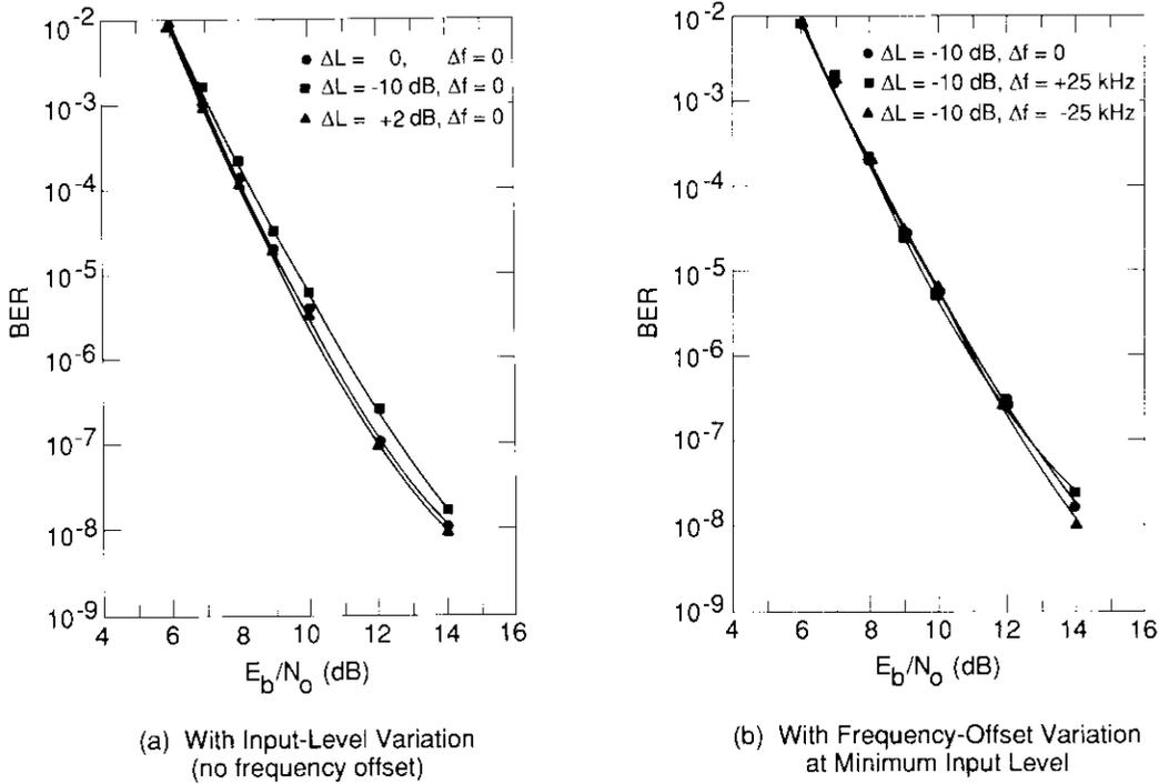
Figure 3. Linear Channel BER Performance Parametric in Receive IF Signal Variations
