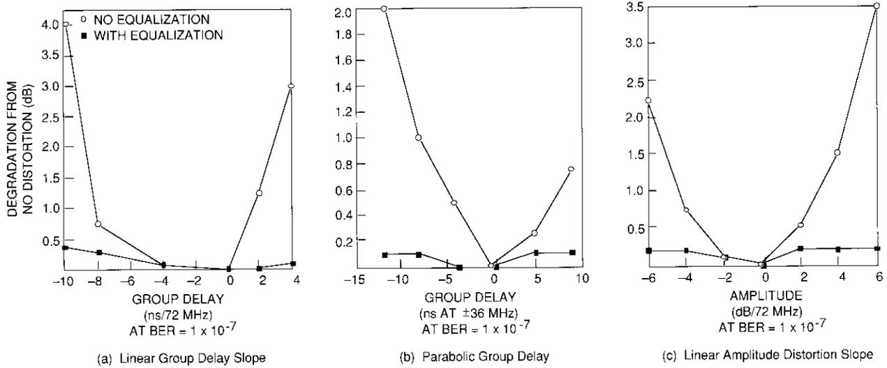
Figure 5. Linear Channel Performance Degradation vs Group Delay and Amplitude Distortion
