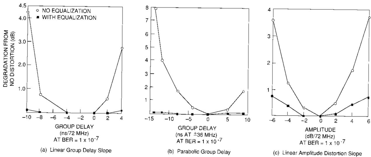
Figure 6. Nonlinear Channel Performance Degradation vs Down-Link Group Delay and Amplitude Distortion
