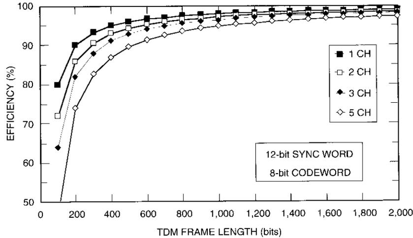
Figure 5. Multiplexer Efficiency
