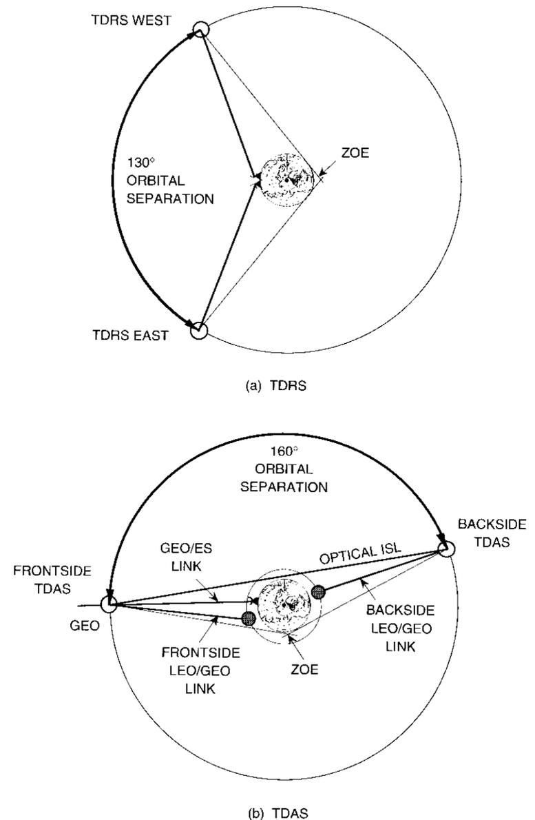
Figure 1. Orbital Positions for TDRS and TDAS
