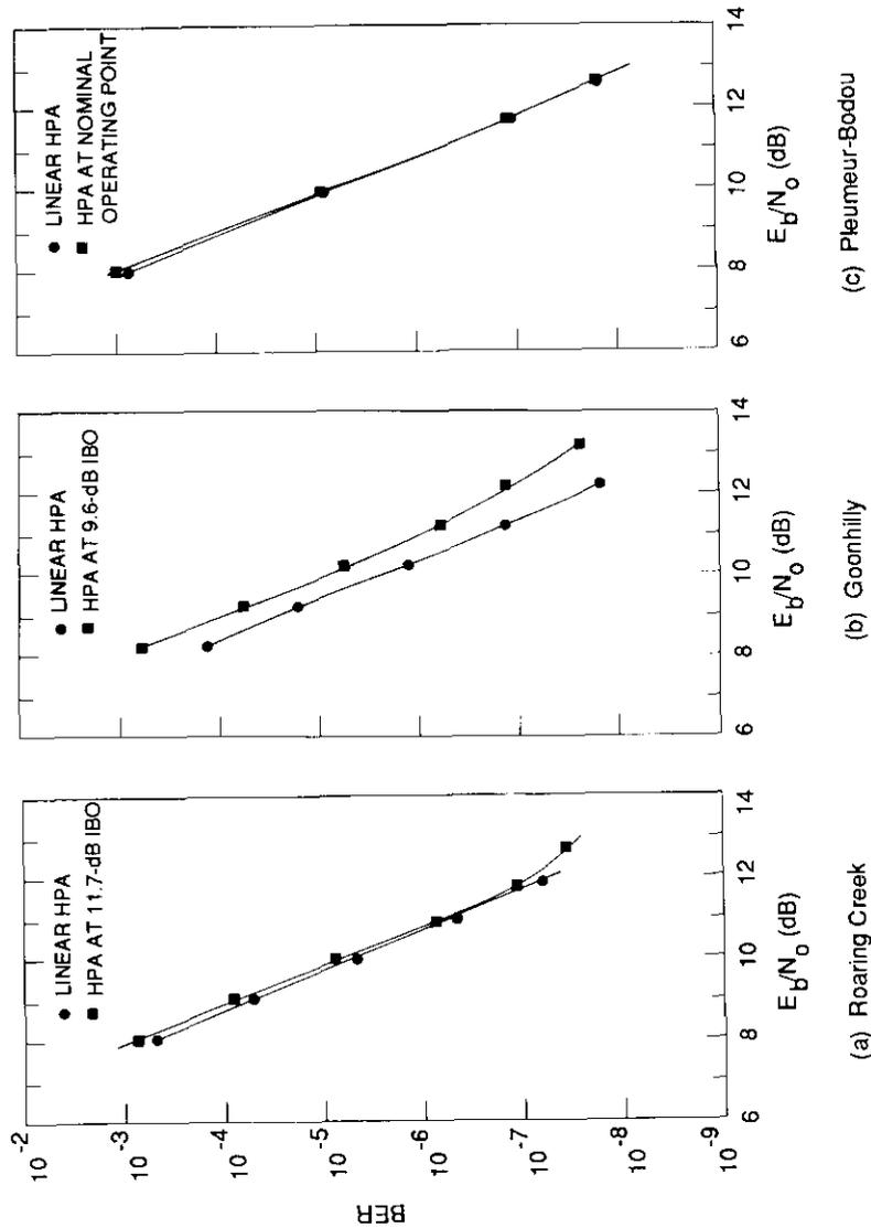
Figure 9. Earth Station Loopback BER vs  $E_b/N_0$
