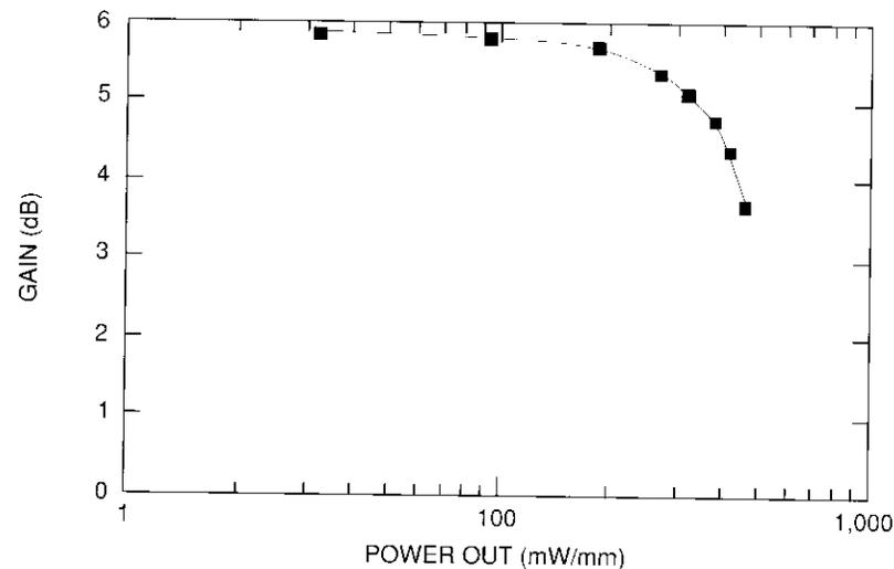
(b) 32-GHz Gain vs Output Power
