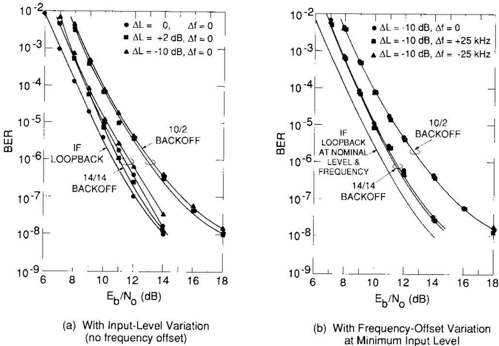
Figure 4. Nonlinear Channel BER Performance Parametric in Receive IF Signal Variations and Transponder IBOs
