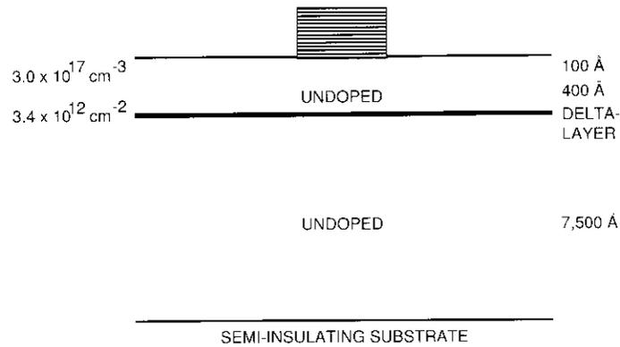
Figure 7. Structure of the Delta-Doped FET
