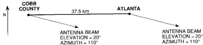
Figure 1. Configuration of the 12-GHz Site Diversity Measurement Near Atlanta, Georgia
